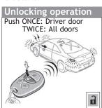
**NOTE:** After unlocking, if a door is not opened within 60 seconds, all doors will relock for safety.
